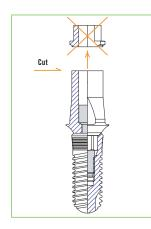
• **The PDT** may be used as a pre-formed abutment with non-frictioning hex, in which case, cut the part indicated in the diagram.
